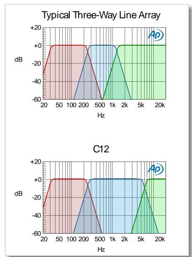
This graph shows the extended bandwidth of the midrange component that is uninterrupted by a crossover point in the critical intelligibility frequency band.
