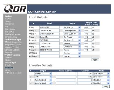
Figure 2-6: Assigning an Output from the list box
