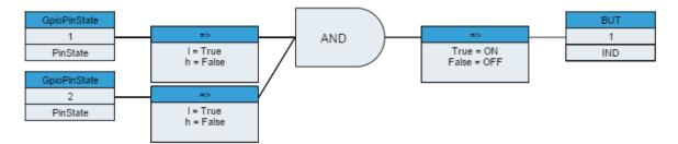
Essentially this flow will light the indicator light on the button only if both GPI 1 and 2 are low. This does not look very useful, but if we were to change the endpoint to be a route destination, it becomes more interesting. To do this, double click on the endpoint box and instead of a GPIO, expand the routers section and select the CurrentSourcePath property of one of the router destinations.
