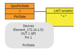
Double click on the ending block and repeat the procedure to select the endpoint or the property we want this flow to change. In this case, I am going to pick an LCD button, but you could also pick a GPO in order to make the GPO state follow the GPI state.
