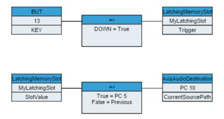
Now the button will cause the latching memory slot to switch back and forth between true and false and if the slot's value is true source PC 5 will be routed to Destination PC 10. If the slot value is False then whatever previous source will be routed back to Destination PC 10.
