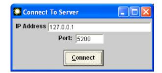
Enter the IP address or fully qualified DNS name for the Pathfinder Core PRO system. For use with Pathfinder Core PRO, the port should always be left at 5200.
