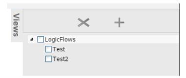
While you can add flows to the master LogicFlows view, it is not recommended as this is the one view that you cannot completely delete. It is recommended that you devise a strategy for your view naming and create the appropriate views underneath Logic Flows to hold your flows. It is also important to note that each view is limited to displaying 100 flows.
