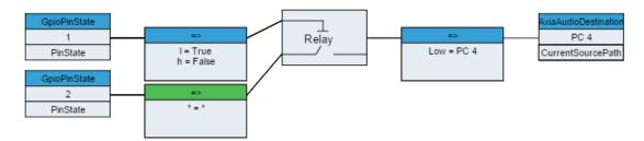
This will actually achieve the same functionality as our previous example, but in a different way. GPI 1 must be low in order for changes taking place on GPI 2 to pass thru. If it is low then changes from GPI 2 will be passed to the output translation which converts the Low to a route change.
