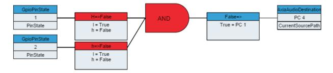
This essentially means a user has to hold two GPIO buttons down simultaneously, and then the PC4 destination will get source PC 1 routed to it. This is a common scenario where we don't want an accidentally bumped button to change the air chain routing so we require two buttons to be held together.
