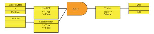
In this case, since the combiner is a logic gate, the translation types are automatically switched to True/False entering and exiting the combiner. By assigning a second GPI pin to the second start point, we can change this event so that two buttons must be held simultaneously in order for the end point change to happen. Edit the various translation lists as described above, and then when complete click apply and you should end up with something like:
