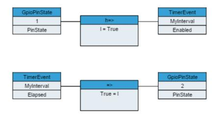
In this case, when GPI 1 goes low, it enables the interval timer. Then the elapsed property 5 seconds later causes GPI 2 pin to be set low.
