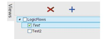
You will notice that once a single view is selected, the Add button (plus) in the main control panel for Logic Flows will switch from its disabled grey to blue indicating that you can now use that control to add a new flow.
