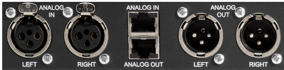
Fig. 1-3: Analog I/O connections
