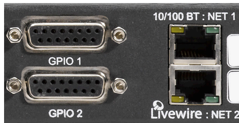
Fig. 1-5: GPIO and Livewire network connections
