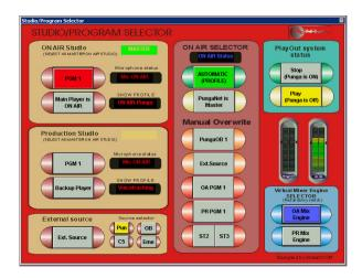
Pathfinder's Panel Designer applet lets you construct custom on-screen controls that can be deployed on PCs across your network. Or, map your custom designed features to rack-mounted button panels and user keys mounted right in the console. Some of these buttons can even dynamically change color and text to display status and engage actions.
