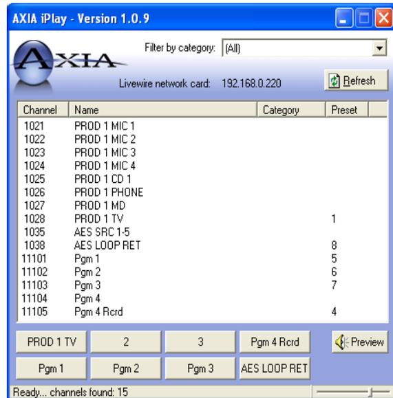
Figure 1-8: iPlay with ACL in effect
