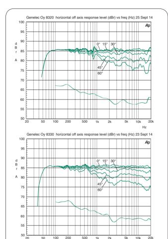
Figure 5: Frequency response plots in horizontal plane of the 8320A and 8330A. The lower curve is the monitor's power response.
