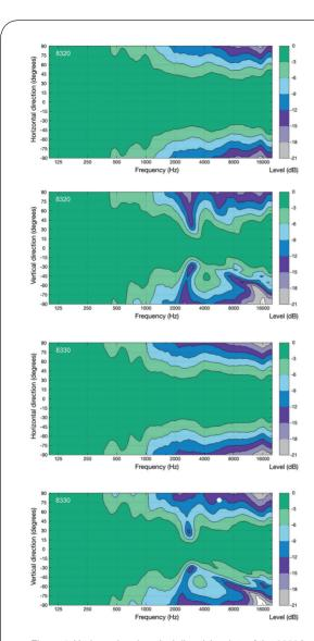
Figure 4: Horizontal and vertical directivity plots of the 8320A and 8330A.
